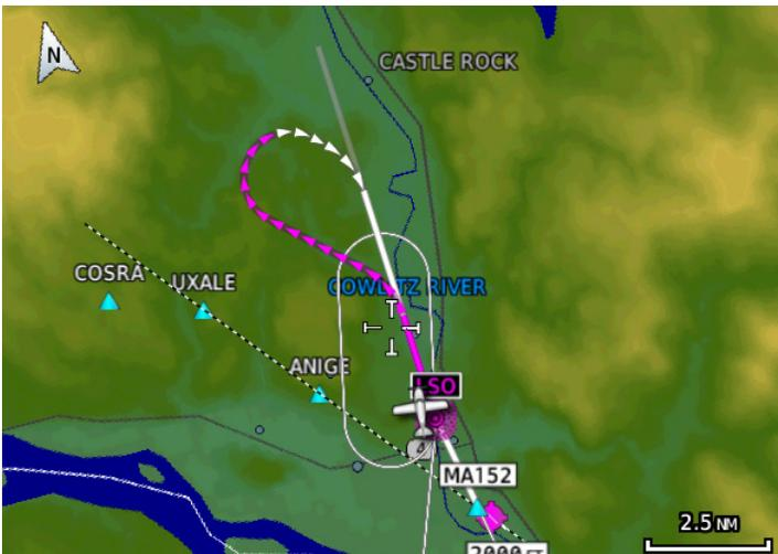
**Figure 8-54 Active Procedure Turn**
