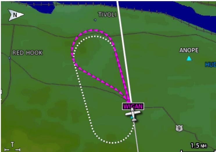
**Figure 8-50 Holding Pattern Entry**
