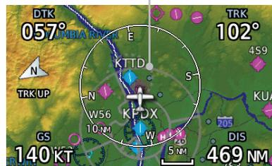
Figure 8-27 Display of Smart Airspaces (Airspace Borders Grayed)
