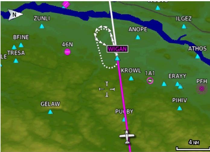
Figure 8-58 Active Flight Plan Leg Prior to Holding Pattern
