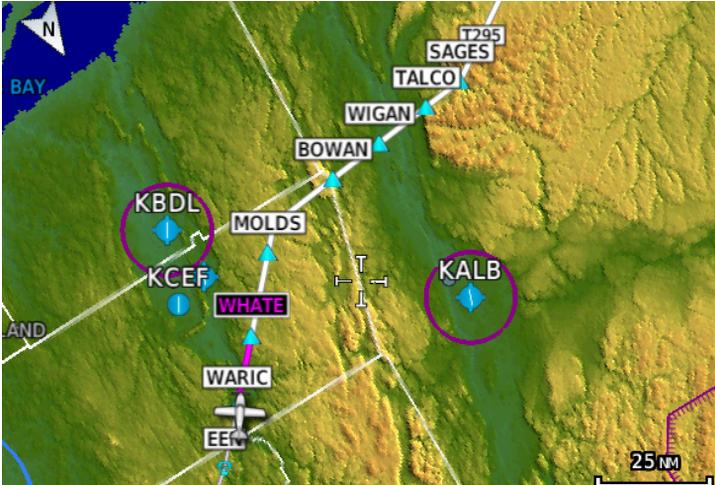
**Figure 8-51 Active and Future Flight Plan Segments**
