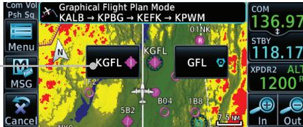
**Figure 8-44 Select the Desired Waypoint From Multiple Waypoints**
