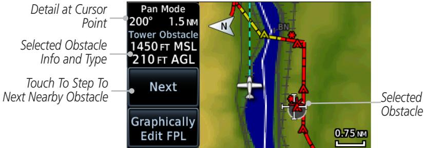
**Figure 8-24 Point Obstacle Detail**
