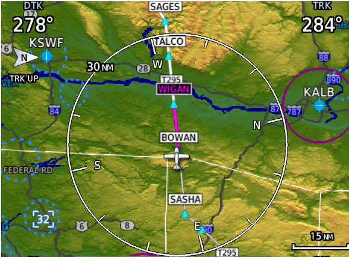
Figure 8-55 Past, Active, and Future Flight Plan Segments
