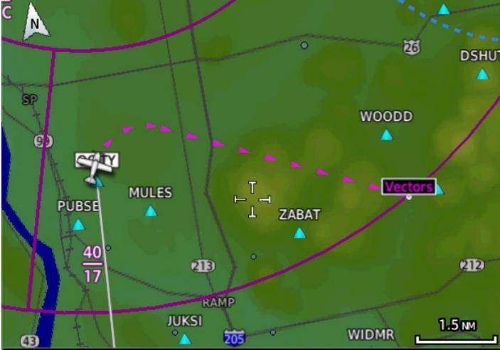
Figure 8-56 Active Heading Leg (Vectors)
