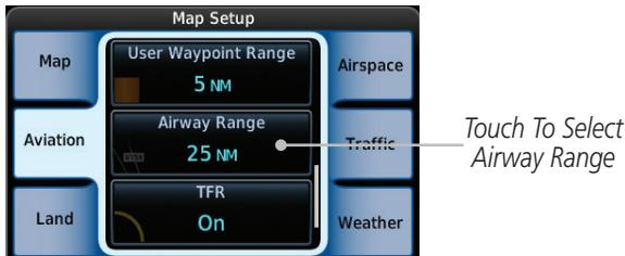
Figure 8-29 Map Setup For Airway Range
