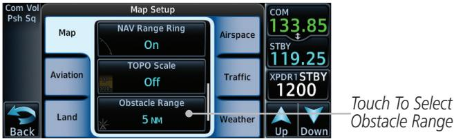
Figure 8-21 Map Setup For Obstacle Range
