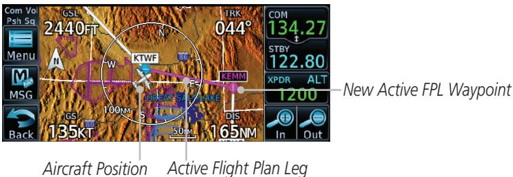
**Figure 8-43 Aircraft Navigates on Edited Flight Plan to New Waypoint**
