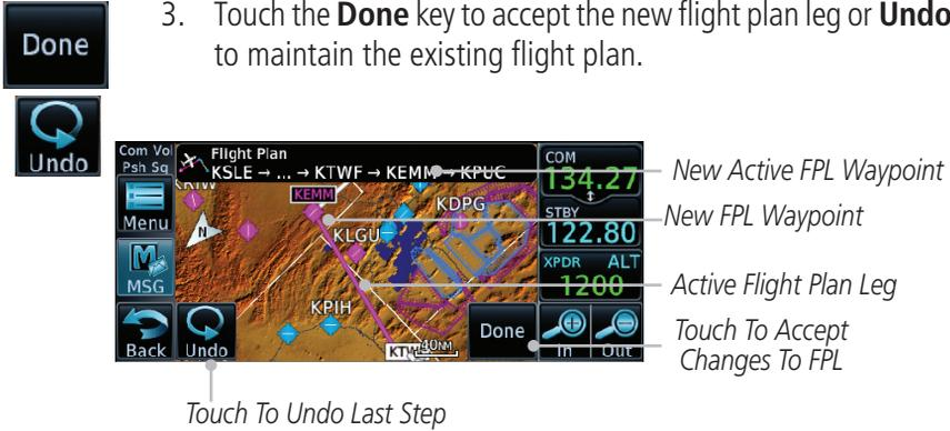
**Figure 8-42 Completed Flight Plan with New Waypoint**
